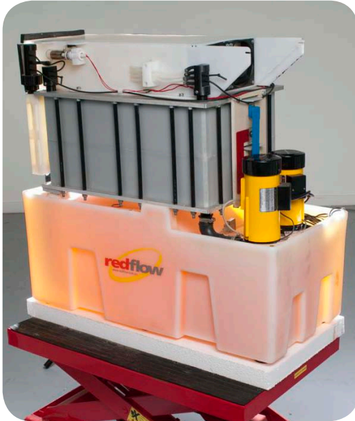
Photo 5. Basic RedFlow ZBM module
